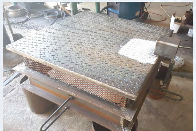
CUSTOM MANHOLE COVER HOLE SIZE 1200X1200MM
