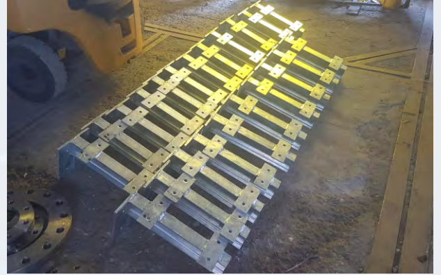
CUSTOM BRACKETS FOR 150NB PIPE
