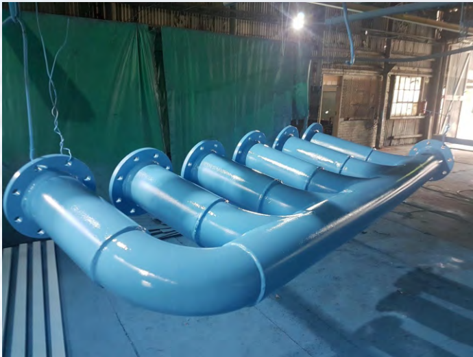
PUMP STATION MANIFOLD ØOPON 891250MIC ARCTIC FROST F28
