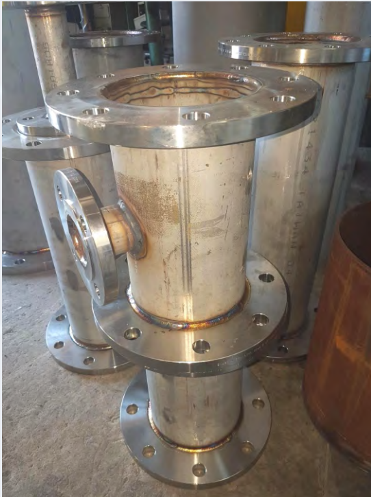
250X80NB TEE FAE T1600/3 GF=280MM
